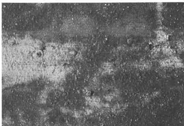
Fig. 3 Detail of the light-red areas showing the roughness of the surface and some of the mechanical damage.
