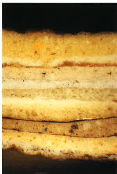
Fig. 8 (above) Cross-section of paint layers on a terracotta by Scheemakers. In all there are about 12 layers.
